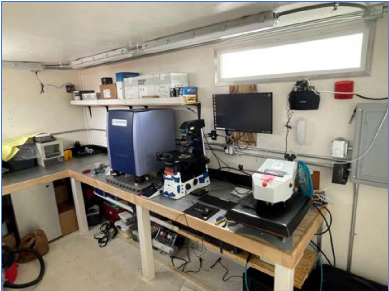
Figure 11. The at-sea genetics and scale lab showing the Fluidigm EP1 (center, tall, blue), the Nikon microscope (just left of the computer screen), and the Knight heat press (right end of the bench).
