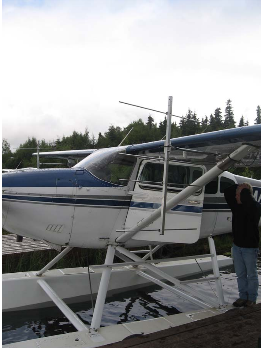
Plate 4. Mounting configuration of 4-element yagi antennas for detecting radio-tagged fish from a Cessna 185.
