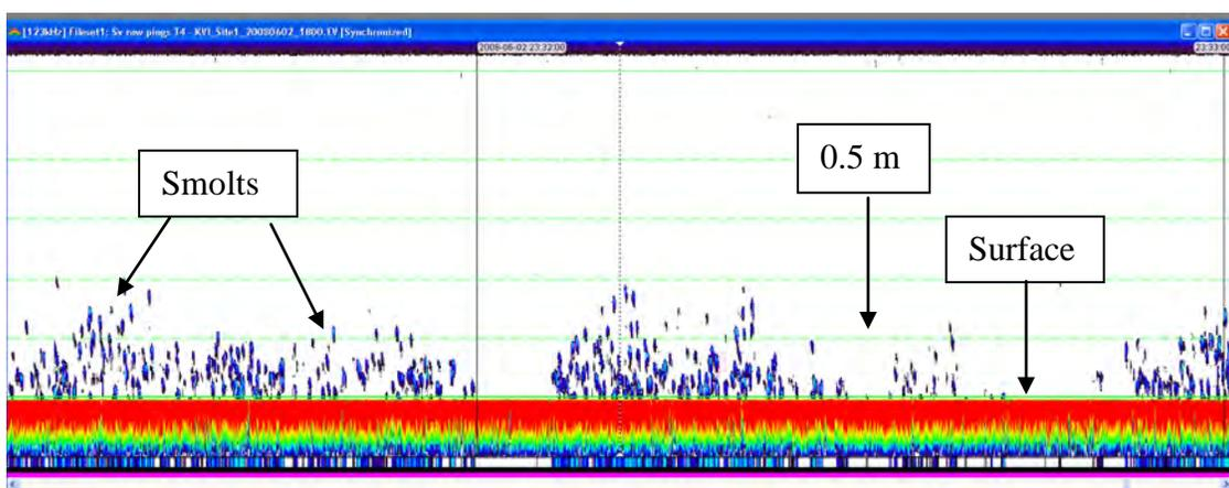
Figure 21. Echogram of smolt detected 2 May, 2008 at Site 1. Dashed green lines signify 0.5 m depth strata and show majority of smolts are in the upper 1.0 m. (EchoView® 4.5 software displays echogram of smolt data as “upside down” due to up-looking transducers.)
