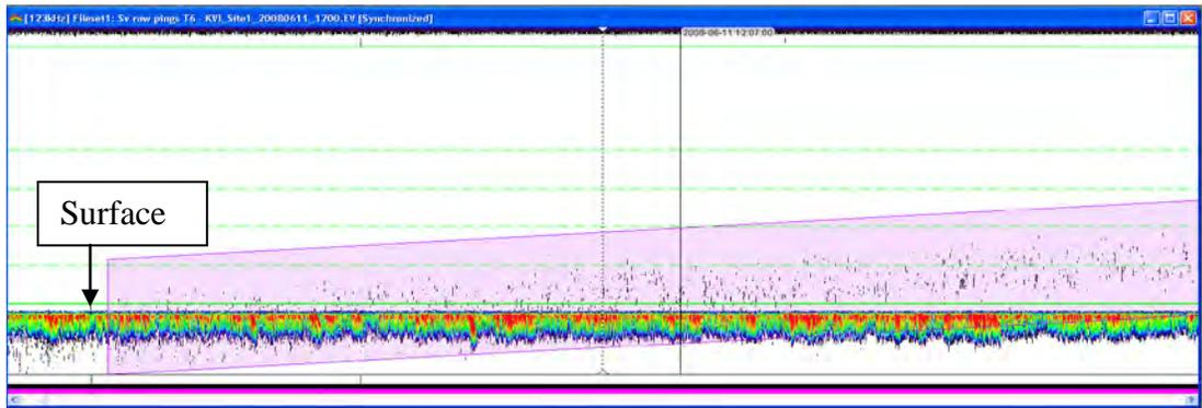
Figure 23. Echogram of cross-talk (shown in highlighted purple region) between transducer six and seven, 2008. (EchoView® 4.5 software displays echogram of smolt data as “upside down” due to up-looking transducers.)
