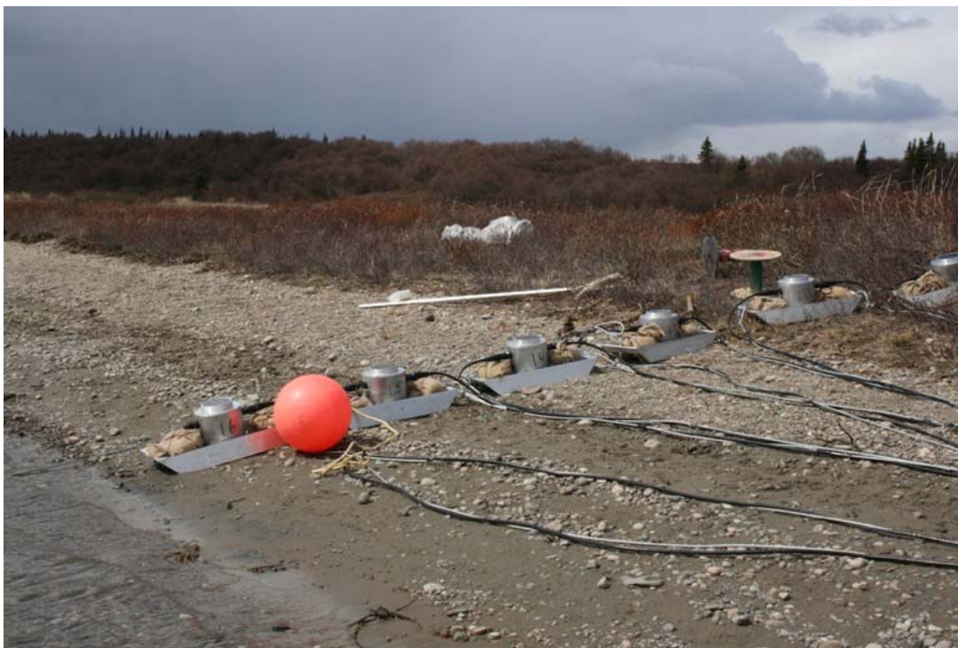
Photo 2. Sonar array of 8 pods prepared for deployment at Site 1 on the river's west bank, 2009.
