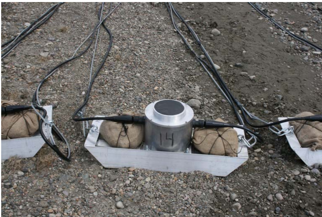
Photo 1. Up-looking transducer mounted on sled with attached power and tow cables used in the Kvichak River, 2009.
